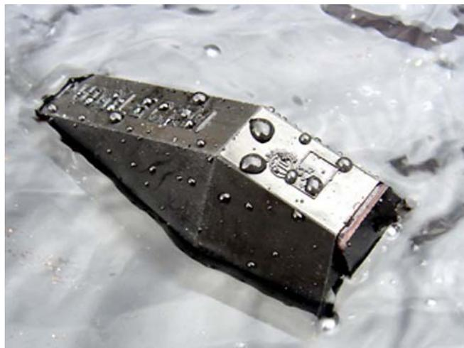
A high-resolution, low-light sensitive single chip camera, giving a resolution of 570 lines, is moulded into a solid acrylic resin housing. For extended life, an option is available with an additional machined titanium housing within the moulding. The plain camera housing is small and indistinguishable, so it can be easily dressed or camouflaged if operation is required within the sight line of other cameras.
