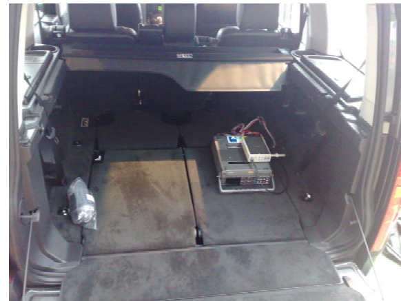
Wide Boot Area Single Recorder Installation Equipment Strapped using integral hooks
